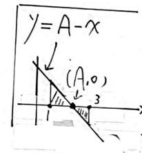
$$f(x) = -x + A \quad \text{③ } 1 \leq A \leq 3 : A = \int_1^A (-x+A) dx + 2 \int_A^3 (A-x) dx \Rightarrow A^2 - 5A + 5 = 0 \Rightarrow A = \frac{5-\sqrt{5}}{2}$$
